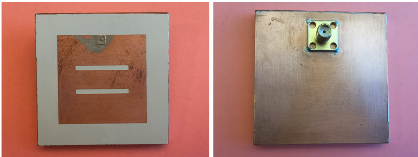
Fabricated slotted patch antenna(with permission from Antenna Lab, WPI)
